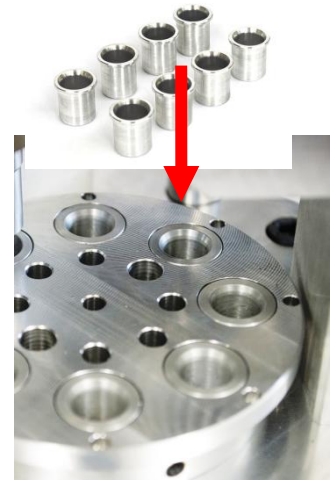
Insert in the drum the case centering bushings
